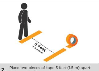
**2.** Place two pieces of tape 5 feet (1.5 m) apart. Distance is critical to system performance.
