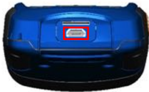
Figure 44: Reveal showing the rear door open and the USB port (for connectivity) highlighted.
